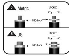
**STEP 5** *Universal Mic Attachment*After choosing desired thread, place microphone on universal mic attachment.
