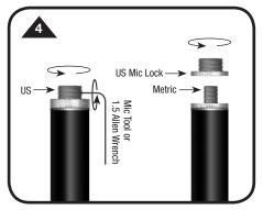
**STEP 4** *Universal Mic Attachment*To adjust US to metric, use tool provided or 1.5 Allen Wrench to unlock threads.
