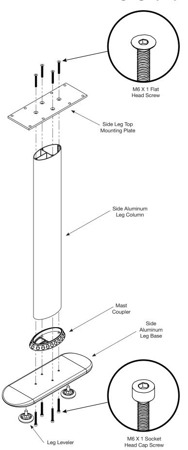
Place side leg top mounting plate on aluminum leg base, lining up the holes. Use the four flat head screws provided to attach plate to leg base. Use M4 hex wrench to tighten flat head screws.
